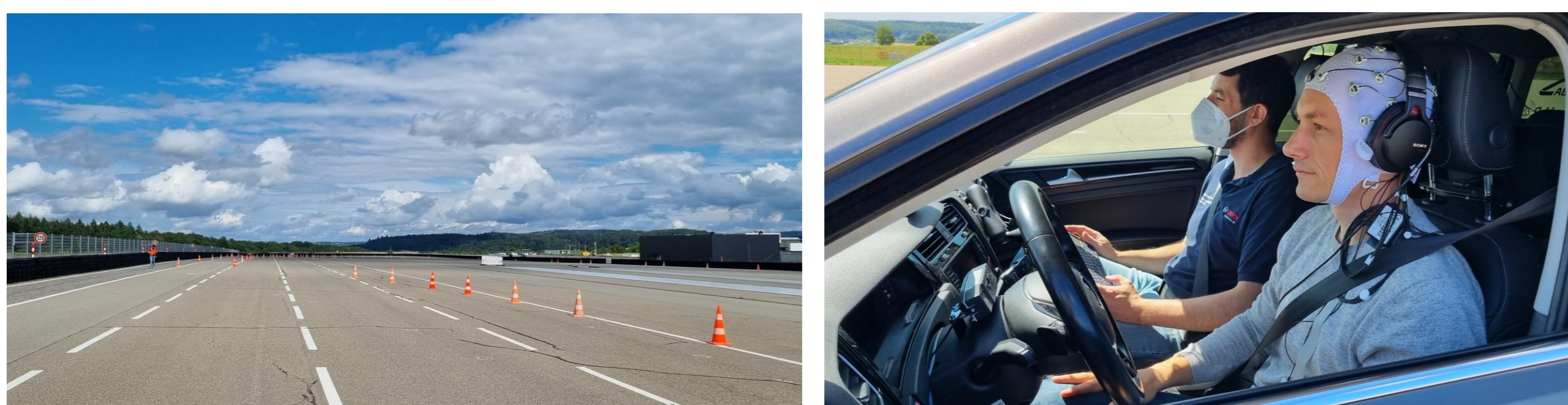
Figure 2 The test track and the vehicle used in the experiment. The participant is wearing a 32-channel EEG cap and headphones for the auditory stimuli presentation.
