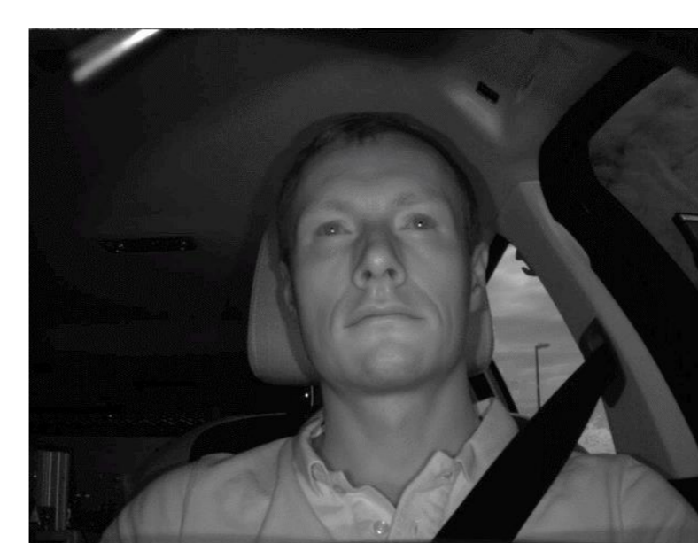
Driver monitoring camera (DMC): ca. 50 x 38° FOV (HxV) 1280 x 960 px 6 x 940 nm Illumination 48 Hz
